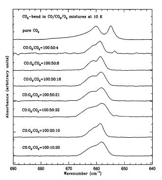
**Fig. 3.** Infrared absorption spectra of the  $CO_2$  bending mode in  $CO:O_2:CO_2$  mixtures. The double structure is evident for pure  $CO_2$  and can be well distinguished in a  $CO:O_2:CO_2=100:50:8$  mixture. When the concentration of  $CO_2$  in the matrix increases, the formation of complexes leads to a general blending.
