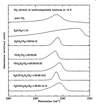
Fig. 2. Infrared absoption spectra of the  $CO_2$  band in multicomponent mixtures. This figure illustrates the strong dependence of the  $CO_2$  stretching mode on the ice composition. When more than a few % of water ice are included in the mixture strong profile changes may occur, as observed for a  $CO_2$ : $H_2O=10$ :1.
