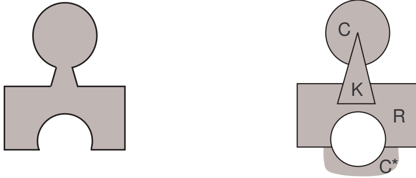
Figure 4: An example of a composed phi-object, C \cup K \cup (R \cap C^*) .
