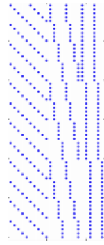
FIGURE 4.3. The sparsity of the Jacobian matrix. The blue points show the nonzero elements of J .
