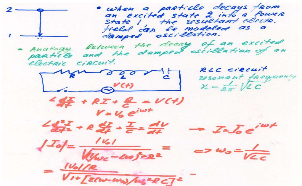
The power w (w) dissipated in the circuit is R/I./2 W = 11/2/R 1+ [2/w-wo)/w22C72 which is a Lozentzian - Shaped resonance CURY WITH FWHM A W=W2RC The quality factor CR of the circuit is defined as  $Q = \frac{\omega_0}{\Delta \omega} = \frac{1}{\omega_0 RC}$
