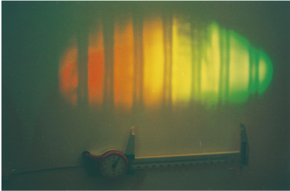
Fig. 4. Image of the SHG of \text{LiF:F}_2^- SSSL 4.3 m away from the SHG crystal in a multifrequency operation without collimation.
